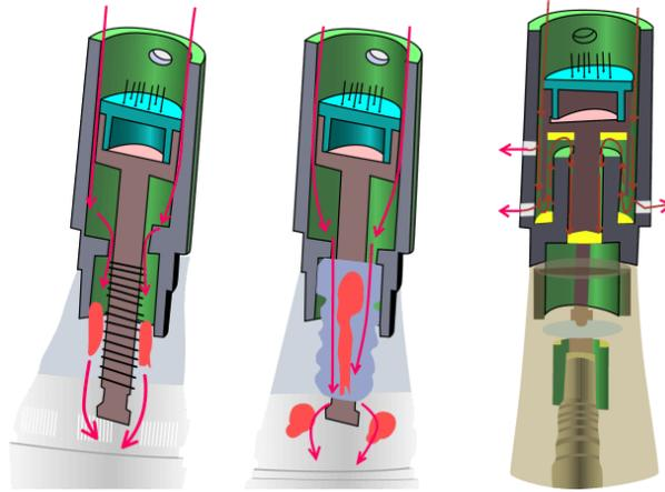
**Metal spring cartridge    Silicone spring cartridge    Biolock cartridge**
